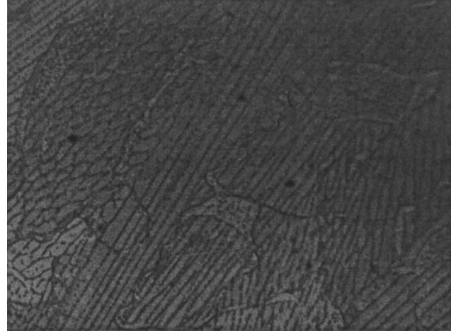
Fig. 4. Cellular precipitation of Pb–Ca–Sn–Ag alloy with inadequate try to fully react with calcium segregated to the subgrain centers (magnification 160 \times ).
